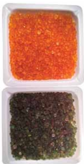
FIGURE 1.6 Silica gel is orange when activated and turns green when deactivated
